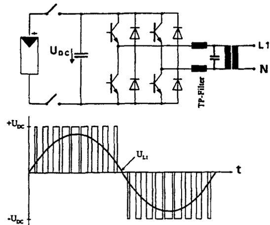
Figure 9.1 The full bridge inverter circuit.
