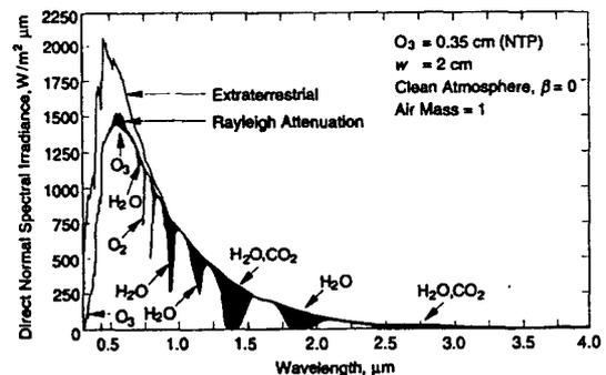
Figure 2.1 An example of the effects of Rayleigh scattering and atmospheric absorption on the spectral distribution of beam irradiance.
