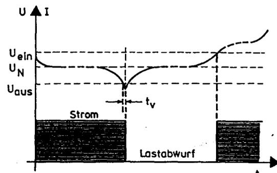
Figure 8.8 Voltage thresholds for deep discharge protection.
