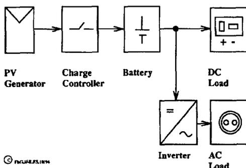
Figure 4.2 Principle schematic of a stand-alone PV power system.
