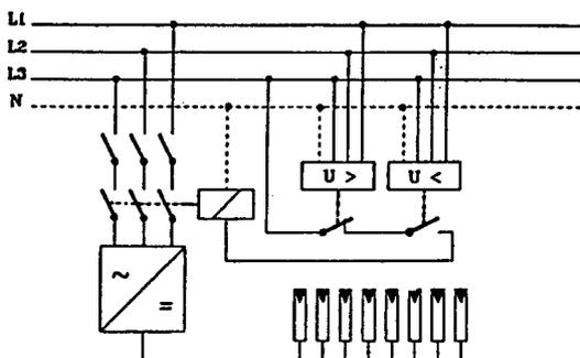
Figure 9.21 Safety concept for a 3-phase inverter PV installation.
