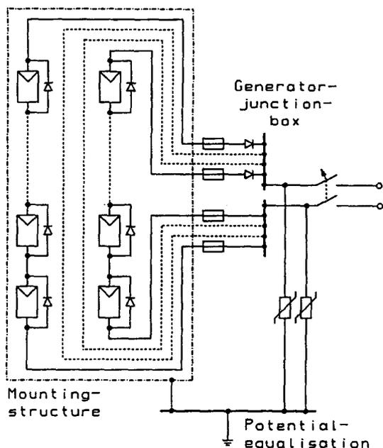
Figure 6.2 Basic structure of a PV generator.
