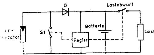
Figure 8.6 Shunt controller.
