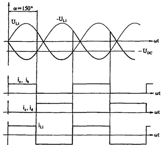
Figure 9.7 Line-commutated inverter.
