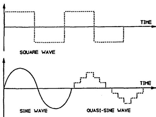
Figure 9.3 Inverter waveforms.
