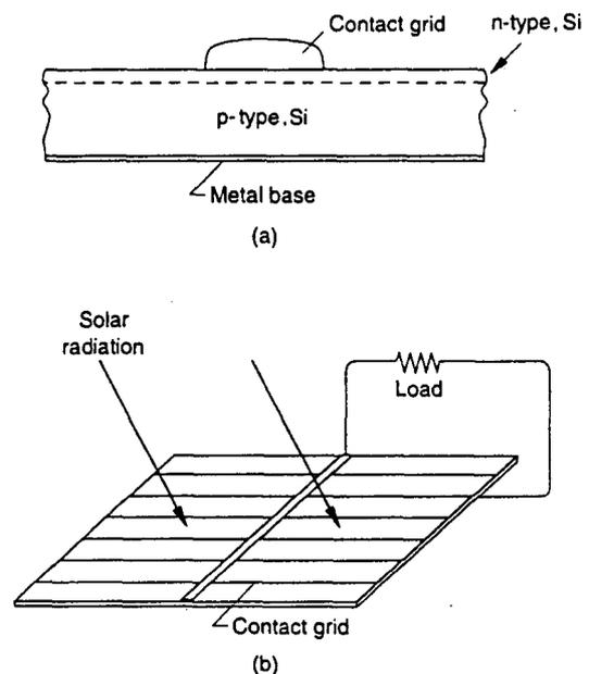
Figure 3.1 (a) Section of a silicon solar cell.
