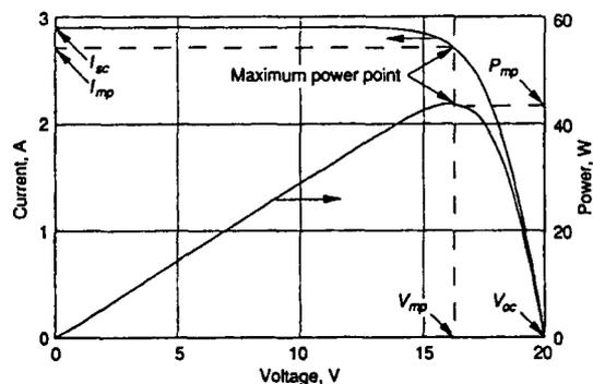
Figure 5.3 I-V curve and characteristic parameters for a typical module.
