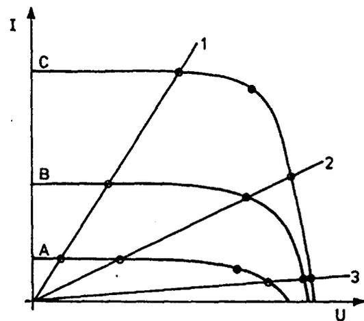
Figure 8.3 IV curves of PV generator, electric fan (dotted line) and three different ohmic loads.
