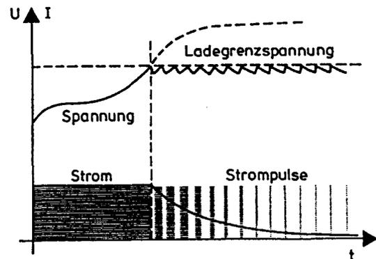
Figure 8.7 Battery voltage and current during charging.
