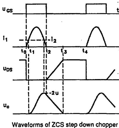
Waveforms of ZCS step down chopper
