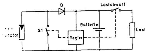
Figure 8.6 Shunt controller.
