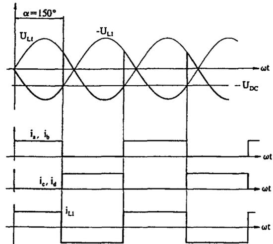
Figure 9.7 Line-commutated inverter.
