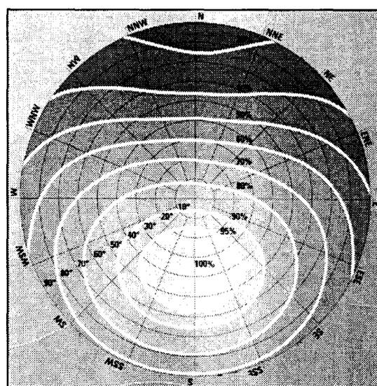
Figure 2.5 Effect of slope (tilt angle) and azimuth (orientation) on the annual incident energy in Central Europe.
